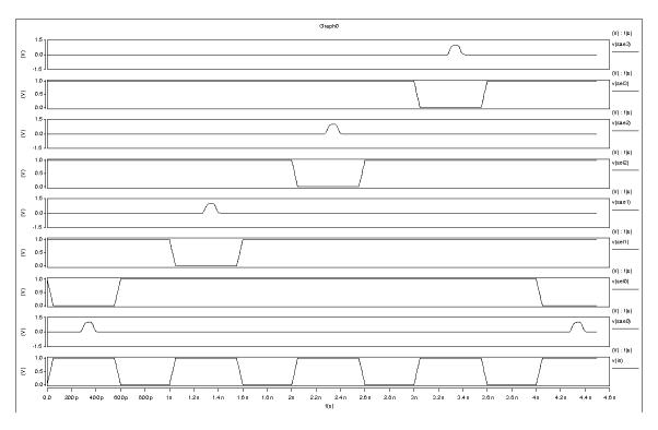
This shows roughly the waveforms obtained for toggling between sel <0> to sel <3> and the obtained sae<0> to sae<3> in pulsed form outputs.
