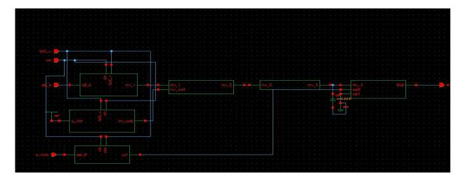
It shows the generation of the GWL as LWL schematic is included in the array picture. The sub-circuits predec\_1b and sel\_inv are used for buffering the lone signals to match their co-ones which pass through NANDs and Inverters and ramp them up to face the desired capacitance. Using Matlab code: the sizes are:
