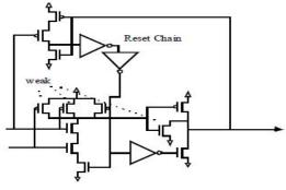
The middle part in the schematic clearly indicates the reset logic. While implementing this logic, the sizing has been taken care to maintain FO4 and to reset accordingly.
