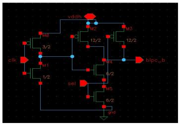
Here an inverter followed by NAND has been used. SAPC generation is almost similar to blpc as it precharges at the same time as bitlines. Only difference in the load capacitance seen by it and hence corresponding sizes of inverter and NAND gate differs. Sel<7:0> varies in the sense that is independent of the clock and is restricted by input capacitance of 24  $\lambda$  on the address input.
